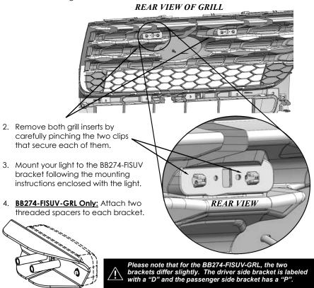
5. Insert the Bracket assembly w/light into the appropriate slot in the front of the grill. Secure it on the backside of the grill with a flat washer, tooth washer, using the screws or threaded studs, as shown to the right.
